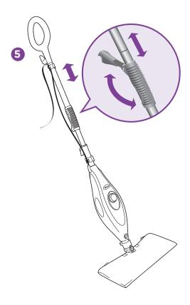
**5** For your comfort, you can adjust the height of the mop. Just lift the latch on the tube 90 degrees to the open position. Holding the handle, extend the tube to the height that is comfortable for you and then lower the latch to locked position.
